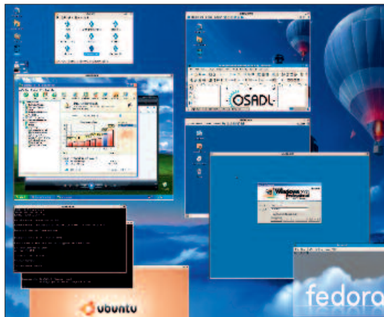
Figure 1. Linux Fedora 7 system running a total of seven virtual systems simultaneously
