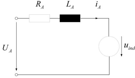
Fig. 3. Equivalent circuit diagram for the permanent excited DC motor.
