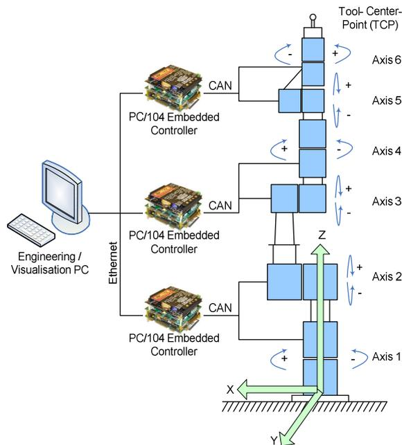
Fig. 6. Embedded Hardware Setup.
