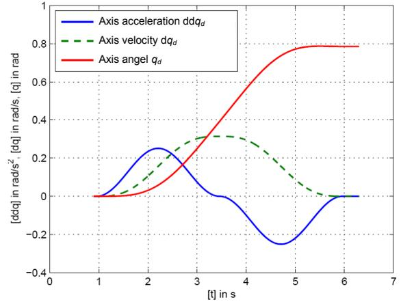
Fig. 5. Trajectory with  $\sin^2$ -based acceleration profile.
