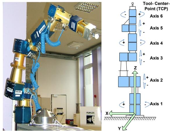
Fig. 1. Mechanical Setup of the Reconfigurable Robot Arm.
