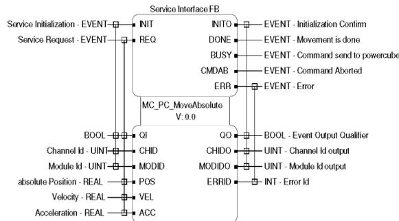
Fig. 8. IEC 61499 Move Absolute Motion Control Block.
