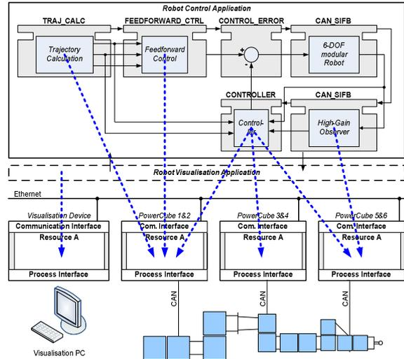
Fig. 7. IEC 61499 System Configuration for the 6-DOF reconfigurable robot arm.
