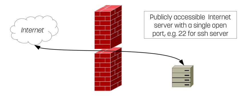
A standard network firewall normally does not protect an active service
