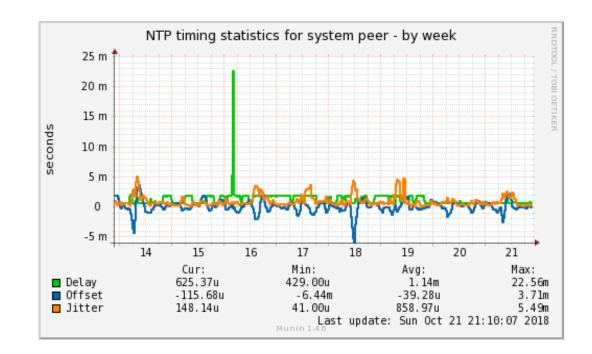
Example of the 1-week time course of the time difference between two NTP-synchronized computers (data obtained from OSADL QA Farm) – Average  $\pm 5$  ms with an outlier of 22.5 ms.
