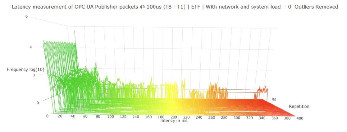
Round-trip time, system under load, **no** real-time configuration
