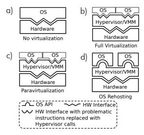
**FIGURE 1:** Overview over different virtualization approaches. Virtualization duplicates the machine interface with high fidelity, whereas paravirtualization replaces problematic instructions with calls to the underlying kernel. OS rehosting goes further and provides a fairly abstracted kernel interface with many implementation specifics left out.
