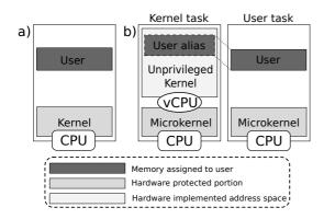
**FIGURE 2:** Implementaion of a subdomain (a) on hardware, (b) on top of a microkernel
