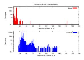
**FIGURE 4:** Latencies in Linux and L4Linux running cyclictest.
